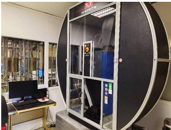
Figure 11 - Examples of impact test pendulums; a) modern computerised equipment, fully enclosed for safety; b) older manual equipment with only partial protection.
