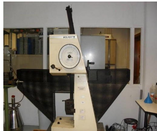
Figure 11 - Examples of impact test pendulums; a) modern computerised equipment, fully enclosed for safety; b) older manual equipment with only partial protection.
